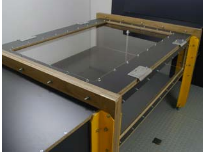
Fig. 5 Test section of 1200x400mm 2D wind tunnel
